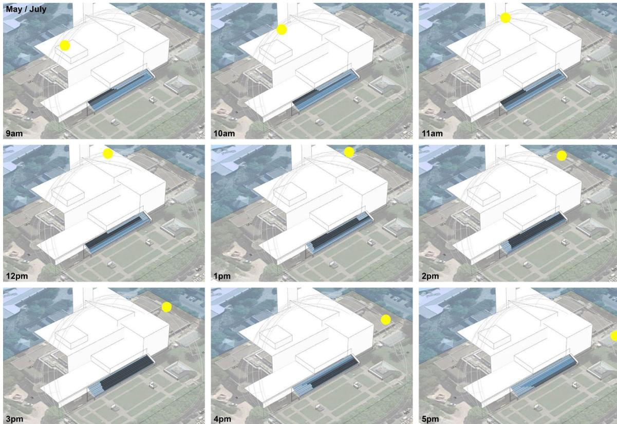
*Fig 12: Geometric Heliotropism - Exterior view on May 21 /July 21 showing glazing tints based on intersections with building forms. Stills from an animation that diagrammed how the skylight would dynamically change over time (Fig 10). Surrounding building massing was included as part of the shading mask, allowing zones of glass occluded by building forms to be untinted.*
