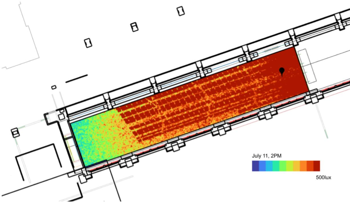
Figure 5A: Point-in-time illuminance at task plane of reading room on July 11, 2 pm (point of peak solar access due to building orientation). Black dot signifies annual sensor data shown in Figure 5B
