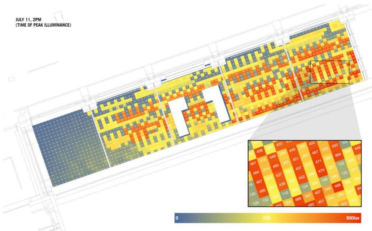
Figure 10: Test calculation with all skylight glazing tinted to 1%, clerestory untinted (60% VLT). Note that the checkerboarding is due to the close spacing of the mullions. Test calculation was performed in Diva4Rhino using materials noted in Table 1 and calculation parameters noted in Table 3 (high-resolution).
