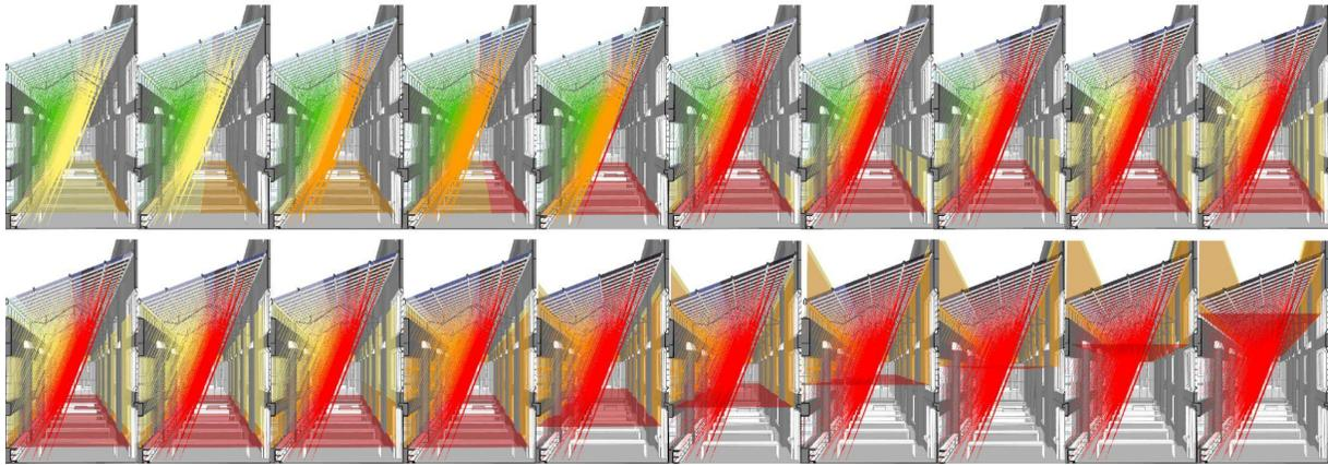
Figure 15: Movement of the jig showing solar vectors for July 11, 2pm. Jig included 45 total steps. Red = 1% tint, Orange = 5% tint, Yellow = 18% tint, Green = no tint (60% VLT).
