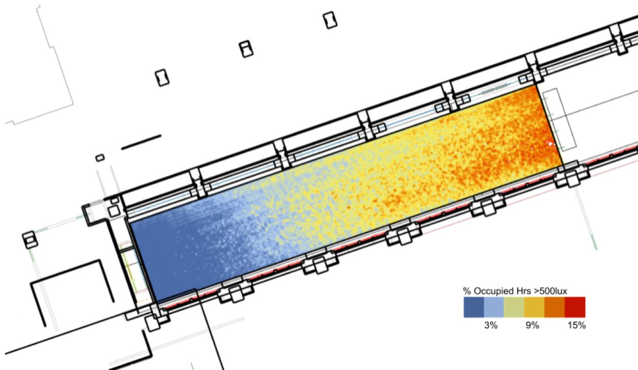
Figure 5C: Percentage of occupied hours above 500lux, calculated using Useful Daylight Illuminance with UDIE set to 500lux (Solemma Climate Studio).
