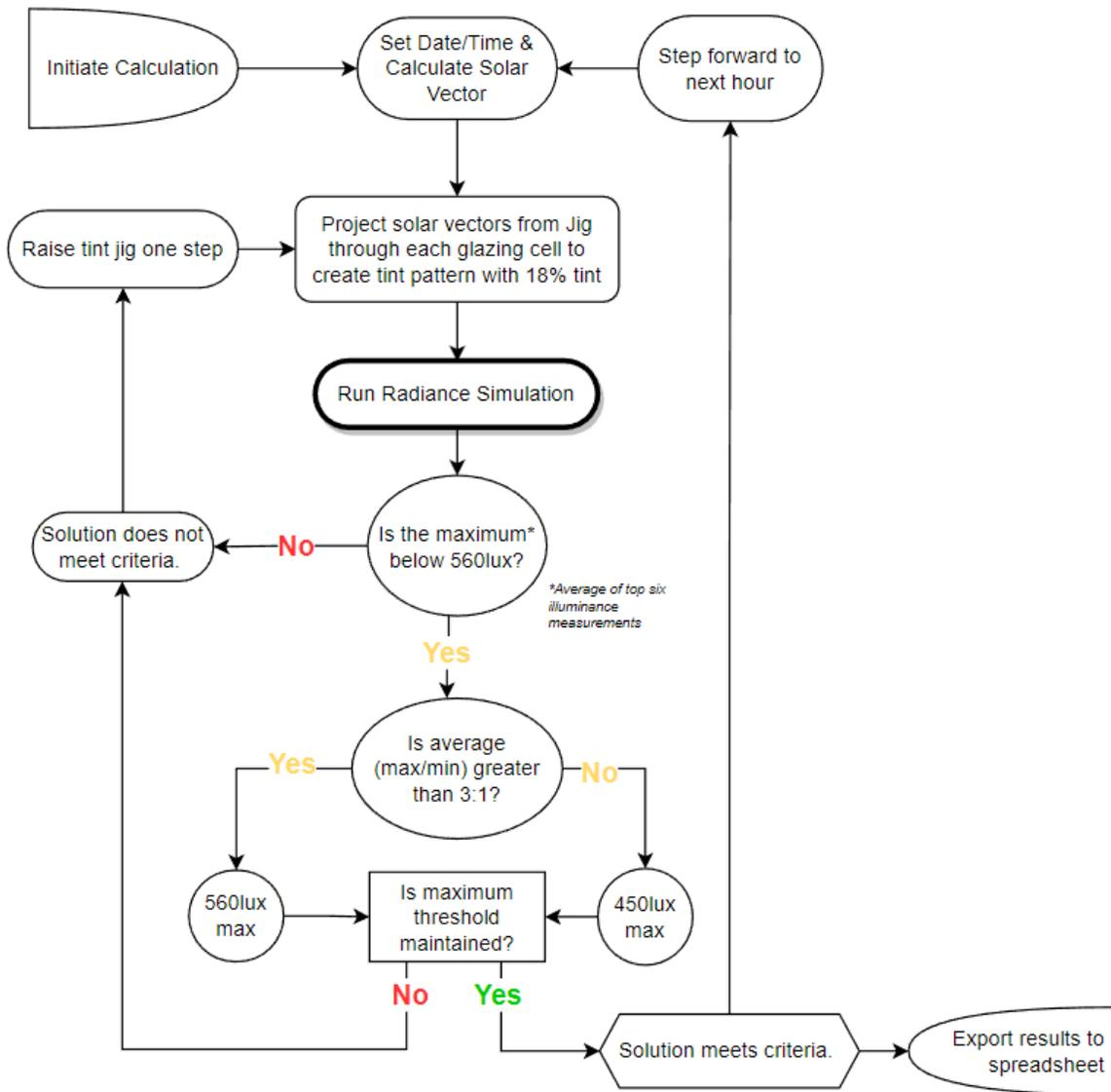
Figure 14: Flowchart explaining the Grasshopper-based looping algorithm for calculating all tint-states.
