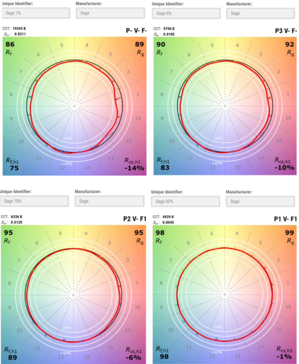
Figure 9: TM-30 color rendition calculations of Sage glazing tints from LBNL Optics6 and processed using IES TM-30 Calculator. This calculation assumes a D65 light source transmitted through the electrochromic material. Data sources include SageGlass\_7\_SR2\_1dk.SAG, SageGlass\_7\_SR2\_6int.SAG, SageGlass\_7\_SR2\_18int.SAG, SageGlass\_7\_SR2\_60clr.SAG
