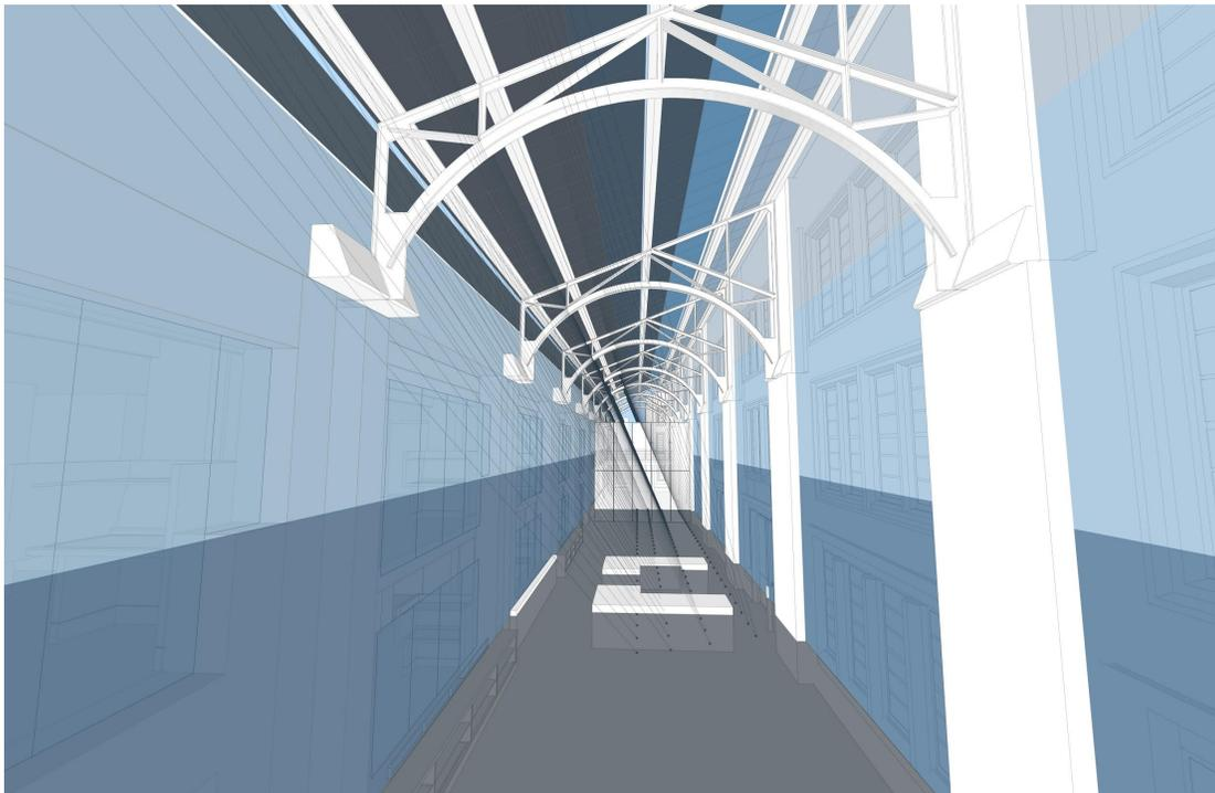
*Fig 11: Geometric Jig. Task plane (dark blue) tints cells to 1% VLT; lower walls (Medium blue) tint glass to 6%, upper walls (Light blue) tint glass to 18%; top of the south wall (Grey-blue) any glass not intercepting rays remains clear.*
