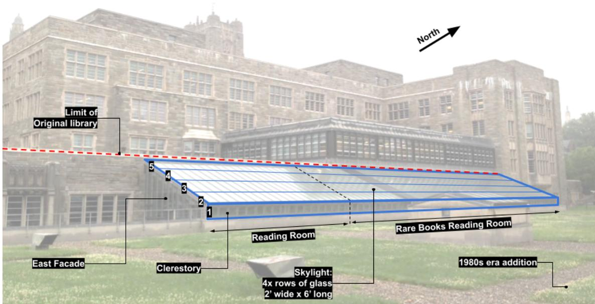
Figure 4. Diagram of the skylight exterior, taken from the roof of the addition before the renovation, showing glazing elements and orientation.
