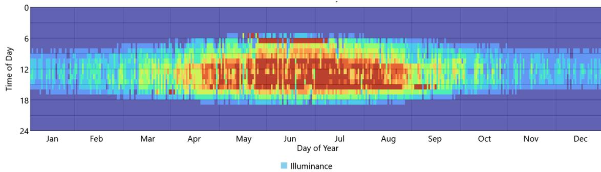
Figure 5B: Daily and Annual Useful Daylight Illuminance at the far-east bay, with the maximum threshold set to 500lux, showing extent of times between April and September when the threshold is exceeded.
