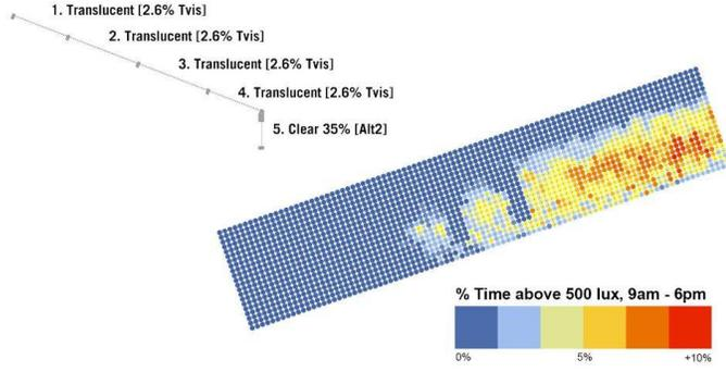
Figure 7: Iteration 2 - various combinations of clear, translucent, and opaque glazing. The annual analysis grid on right shows the percent of hours above 500lux, showing that only the first option would comply. However, the solution would create overly-gloomy visual conditions on the interior. The second option presented an early electrochromic solution for only a single band of glazing.
