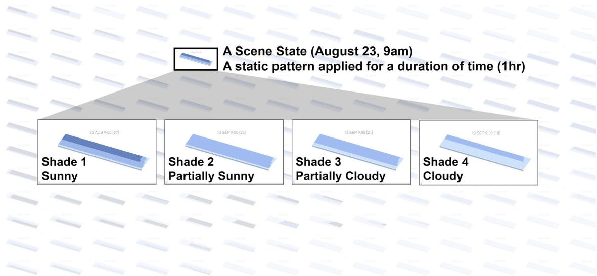
Figure 16C: At any given time, four tint-states are available to account for weather conditions
