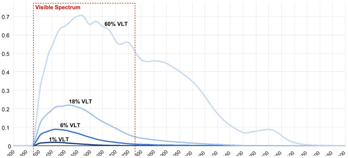
Figure 8: Spectral Power Distributions of the four tint states in Sage Glass. The red outline represents the visible spectrum from 380-780nm. Data sources: LBNL Optics6 including SageGlass\_7\_SR2\_1dk.SAG, SageGlass\_7\_SR2\_6int.SAG, SageGlass\_7\_SR2\_18int.SAG, SageGlass\_7\_SR2\_60clr.SAG
